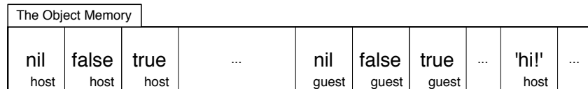
Figure 3. Objects from the host and guest are mixed in the object memory. In this figure, after the nil, true and false host instances, follow the corresponding ones of the guest, which can in order be followed by objects of the host, like the string ‘hi’.
