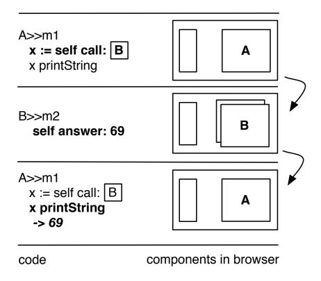
Fig. 3. call:/answer: the basic elements of control flow in Seaside. The framed B in the method m1 is a graphical object displayed as the window B in the web browser. m2 is a method that is invoked in a callback *i.e.*, when an action on the component B is invoked such as a button pressed or a link clicked.
